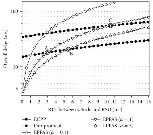
FIGURE 3: Delays of the three protocols with respect to the RTT between a vehicle and the RSU. The RTT between the RSU and the TA is determined by multiplication of  $\alpha$  to RTT between the vehicle and the RSU.
